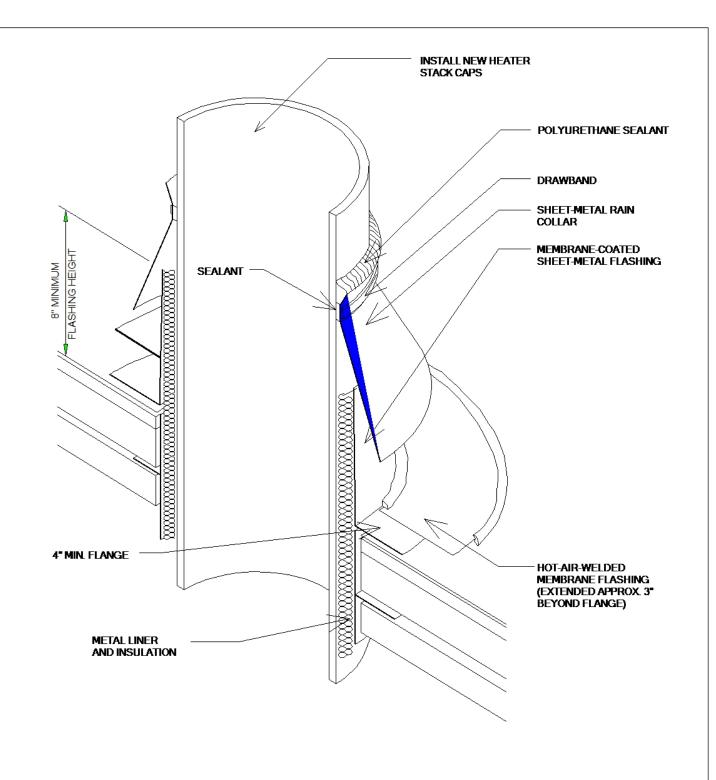
SHEET METAL STACK FLASHING
