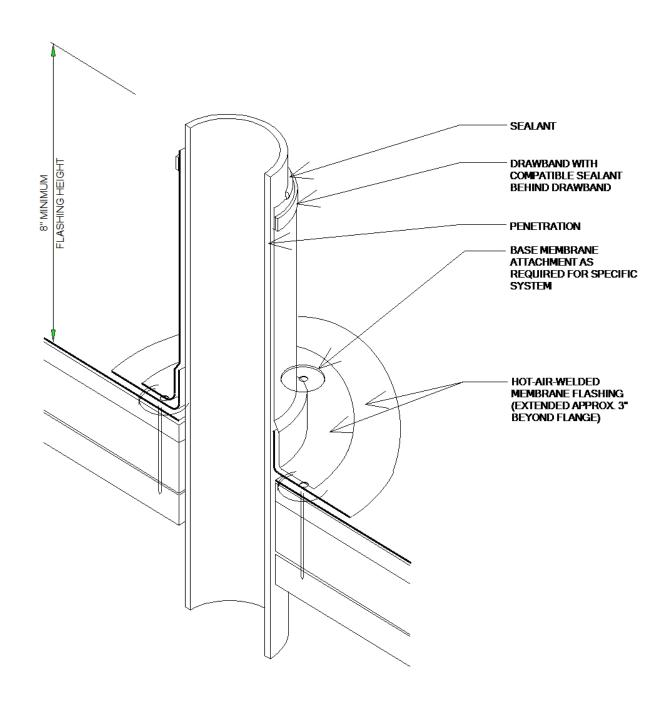
PENETRATION FLASHING [FIELD WRAP]
