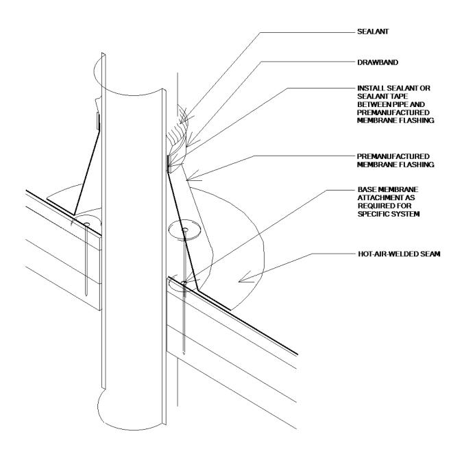
PENETRATION FLASHING [PREMANUFACTURED BOOT]
