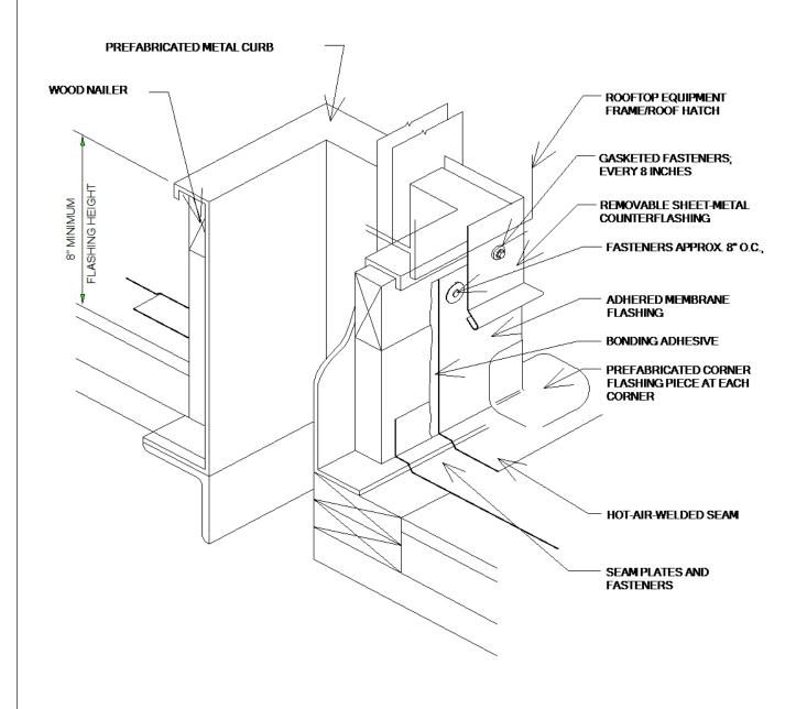
BASE FLASHING AT PREFABRICATED METAL CURB
