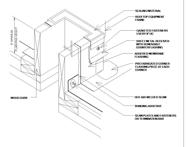
**BASE FLASHING AT WOOD CURB**
